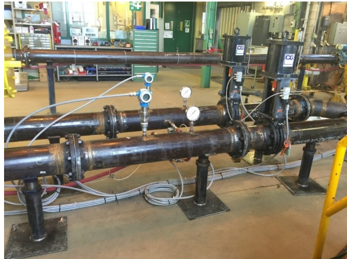
Figure 3 CGIS Alberta Innovates technology futures slurry test loop (AITF) courtesy of author
