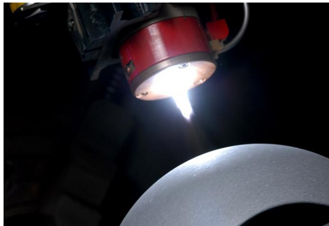
Figure 6 Plasma spray of ball component (courtesy of ValvTechnologies)
