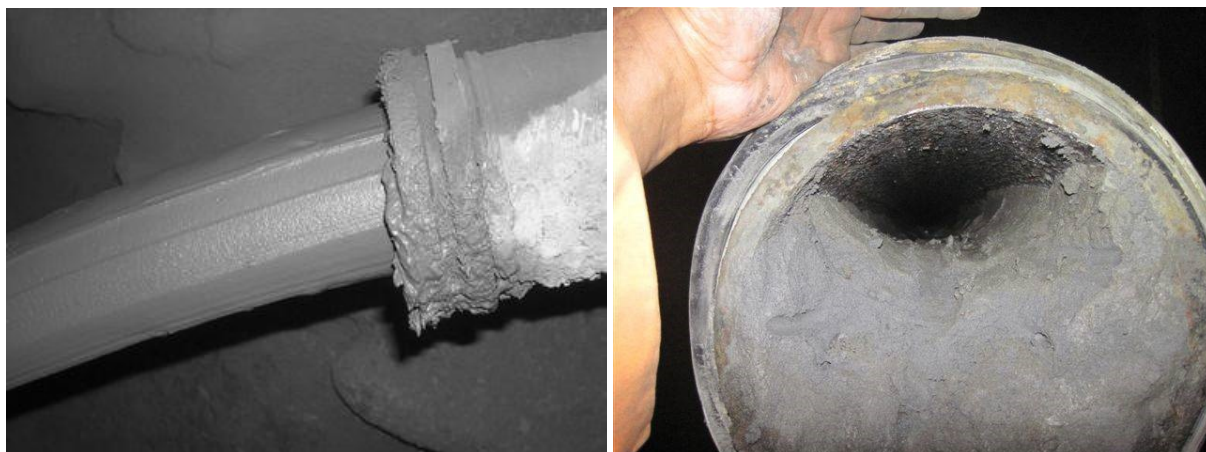
Figure 7 Paste flowing versus paste solidified in the pipeline
