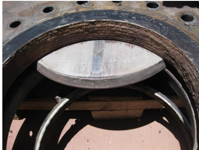
Figure 4 A six-month examination of tungsten carbide weld overlay and gate, showing no measurable wear on acidic tailings (BHP)
