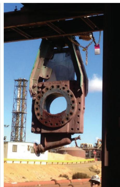
A push-through that consistently provided one to two months operational life (with its discharge collection piping) being removed for the test of a guided shear gate
