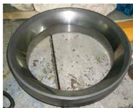
Figure 8: Coated and Mate Lapped Loose Seat Component]
