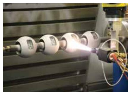
Figure 6: HVOF RiTech® Coating of Ball Component
