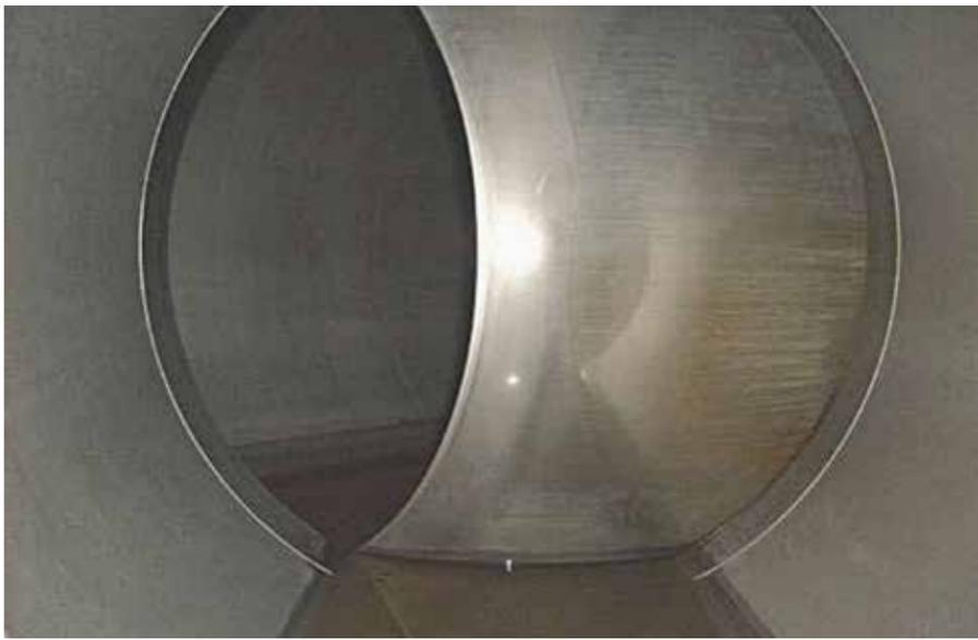
Figure 9: Internal View of Ball Valve Showing HVOF Bore Coating]
