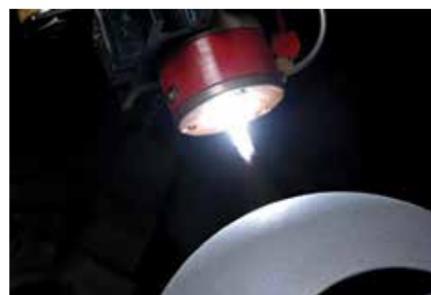
Figure 7: Plasma Spray of Ball Component
