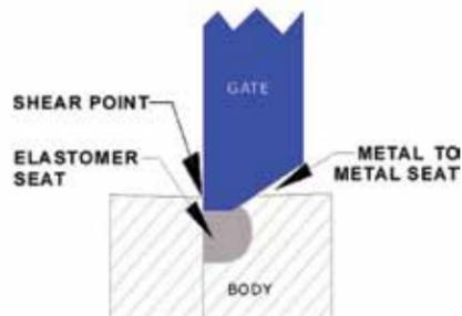
Figure 2: Shear Point and Bottom Sealing
