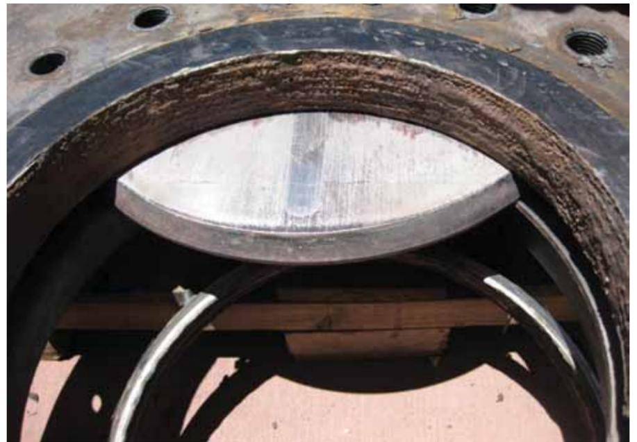
Figure 4: 6-month examination of tungsten carbide weld overlay and gate, showing no measurable wear.]
