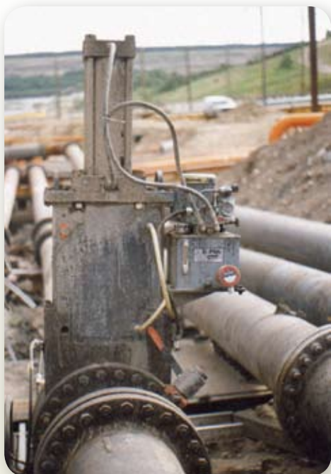
The World's first true ASME Class 300 Knife Gate Valve
